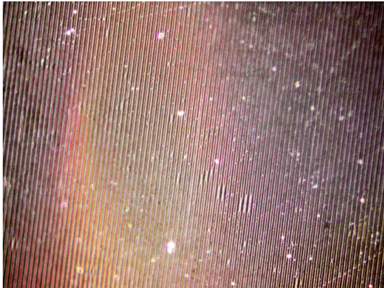
Figure 3.1: Microscopy picture of a type-II PPKTP crystal. The surface has been etched with HF to achieve a contrast in the height of the domains.
