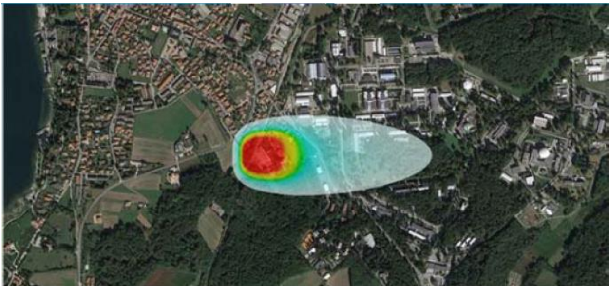
Figure 37. Toxic dispersion from a catastrophic rupture of a tank wagon containing sulphur dioxide.
