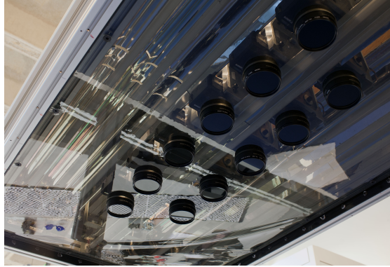
Figure 4.13: Detail image from the acquisition head, showing the acquisition system (11 cameras) and the lighting system (8 fluorescents, reflectant system and polarizer film).
