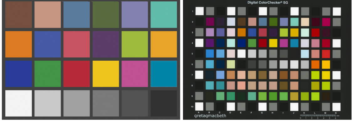
Figure 2.3: Color Checker. The Gretag Macbeth ® color checker chart and the Digital Color Checker. SG ® chart
