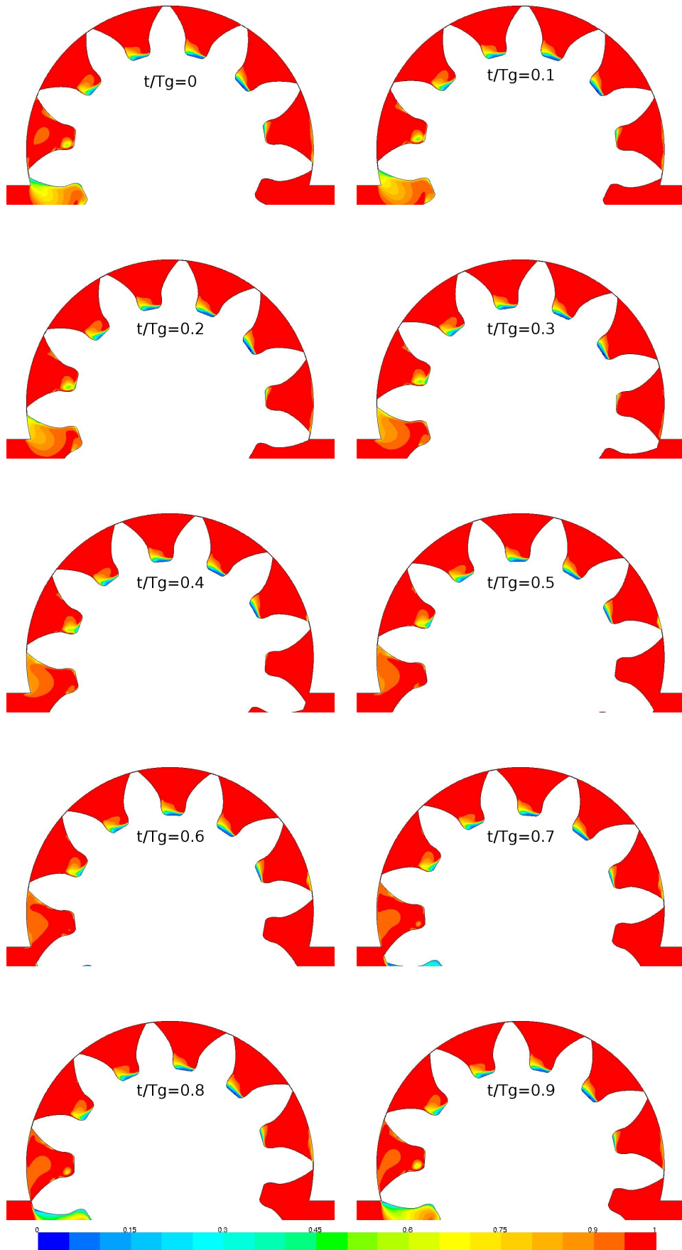
Figure 6.34: Volume fraction of oil trapped between the teeth and the casing at 3000 rpm each 1/10 of a gearing cycle with a pressure inlet loss factor.
