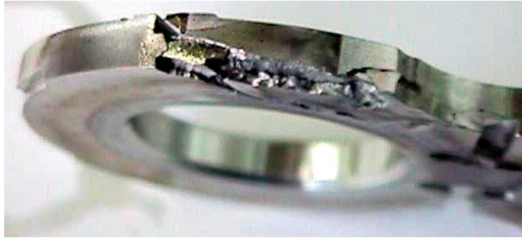
Figure 2.3: Cavitation damage on the compensation plate on an external gear pump.
