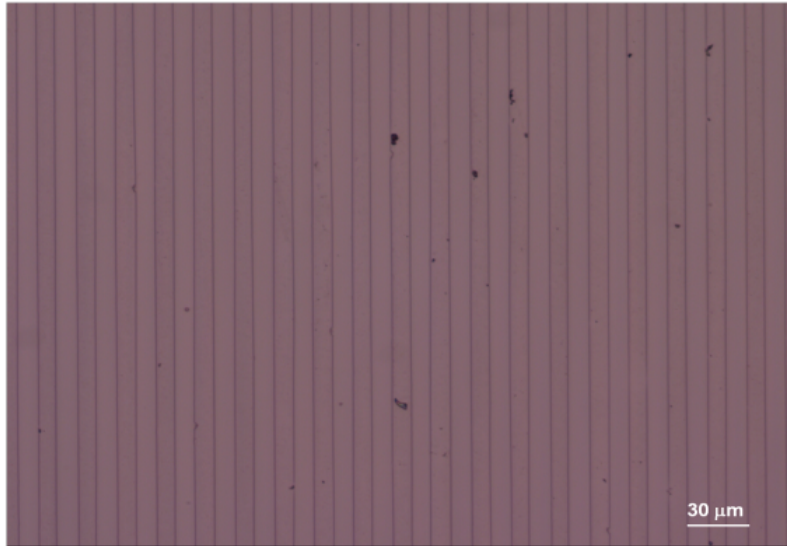
Figure 3.11: Microscope image of a sample of fabricated PPLN after etching.
