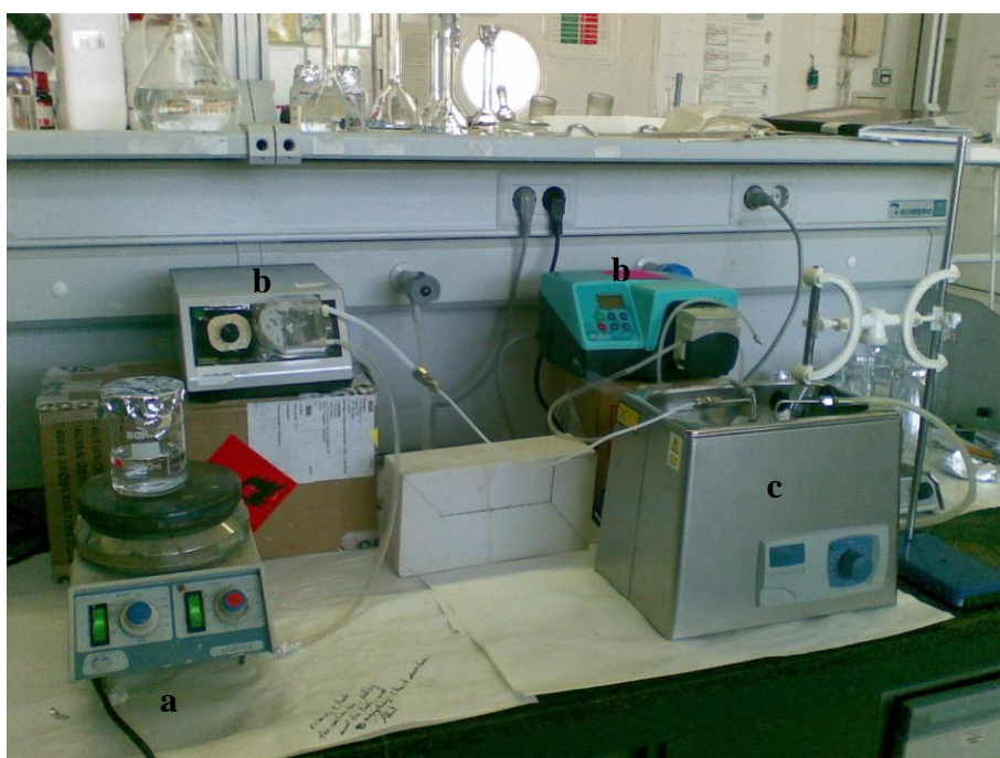
Figure 2.3: Microsystem set-up photo: a- mechanic heaters, b- peristaltic pumps and c- the microreactor immersed inside a Bandelin Sonorex ultrasonic bath.
