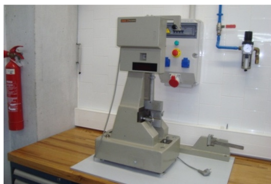
Figure 2.18 Impact testing machine used for the determination of the impact strength of the prepared thermosets.
