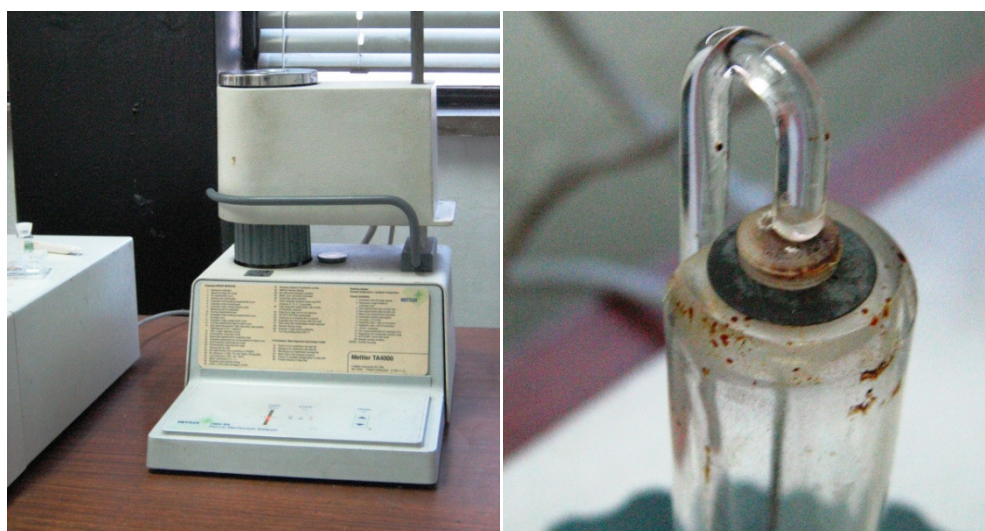
Figure 2.6 TMA apparatus used to perform thermomechanical analysis and magnification of the analyzing probe.
