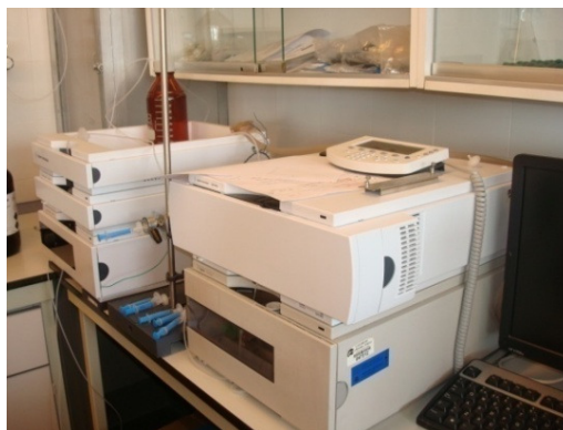
Figure 2.17 Agilent chromatograph used for the molecular weight determination of HBPs.
