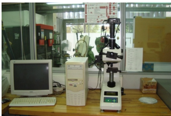
Figure 2.19 Microhardness tester used for the determination of the Knoop hardness of the prepared thermosets.
