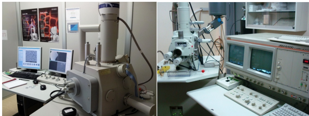
Figure 2.14 ESEM (left) and SEM (right) equipments used for obtaining surface images.
