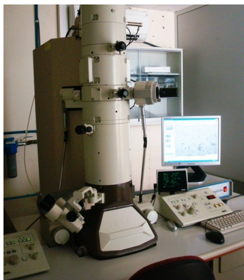
Figure 2.15 TEM equipment used to observe the morphology of the thermosets prepared.
