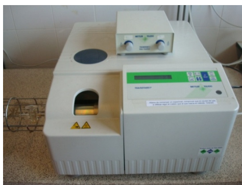
Figure 2.12 Thermobalance used for the thermal stability evaluation.
