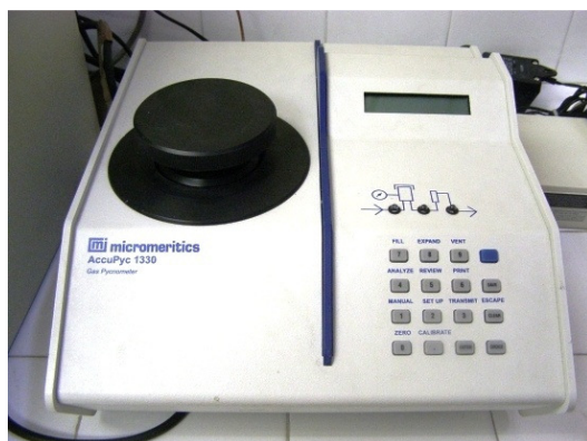
Figure 2.13 Gas pycnometer employed for the density determination.
