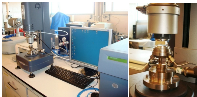
Figure 2.10 Rheometer ARG2 used, with a magnification of the geometry used.
