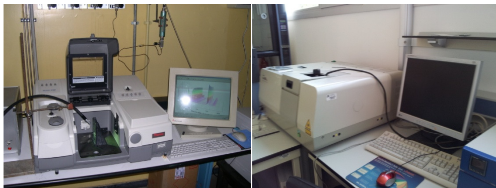
Figure 2.4 IR devices used for photoinitiated (left) and thermal (right) systems.
