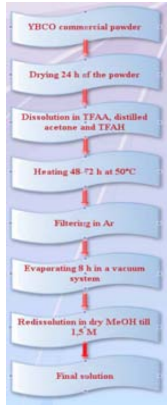
Figure 4.1–1 Synthesis of the YBa_2Cu_3O_{7-x} solution.
