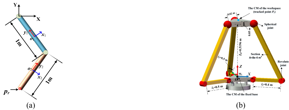
Fig. 1 Two types of robot multibody models. (a) The model of plane serial manipulators. (b) The model of a space parallel delta robot.
