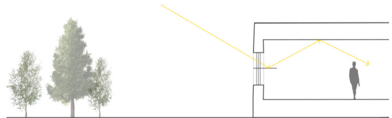
Diagram 12.2 The light shelf reflects light to the ceiling and deeper into the space.
