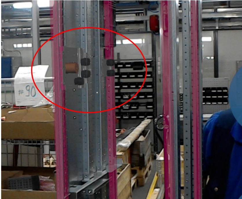
Figure 17. A capture of the view through the HMD. Virtual objects representing the parts to be assembled are shown inside the red circle.
