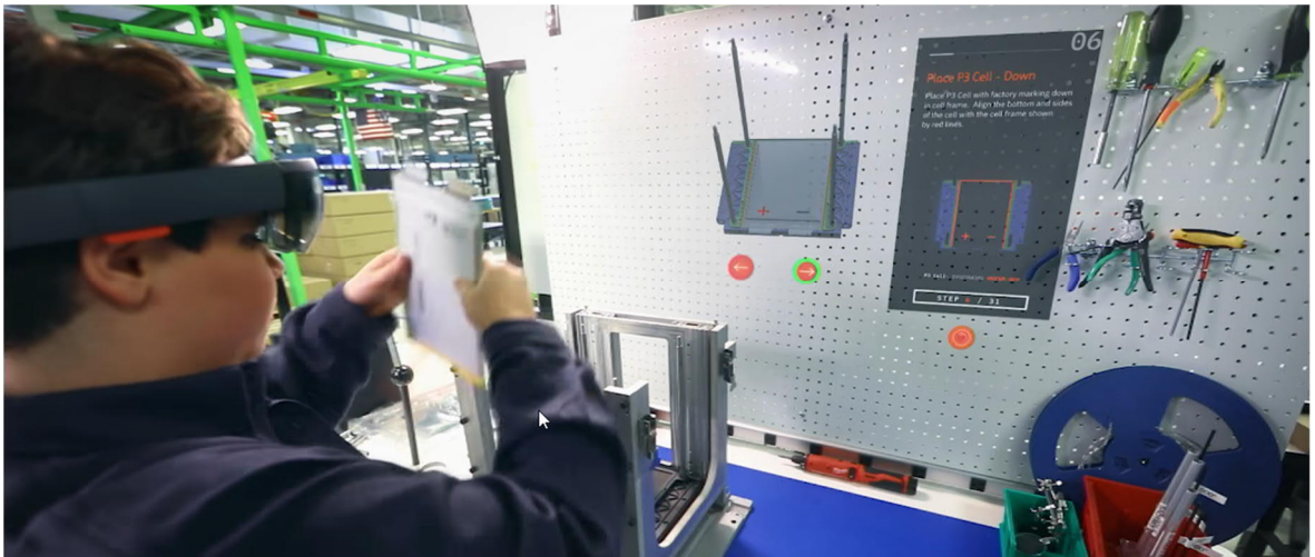
Figure 8. An operator wearing HoloLens. There is a 3D instruction overlaid on the front of the workplace wall. Next to it on the right is a textual description of the task. (PTC, 2018).
