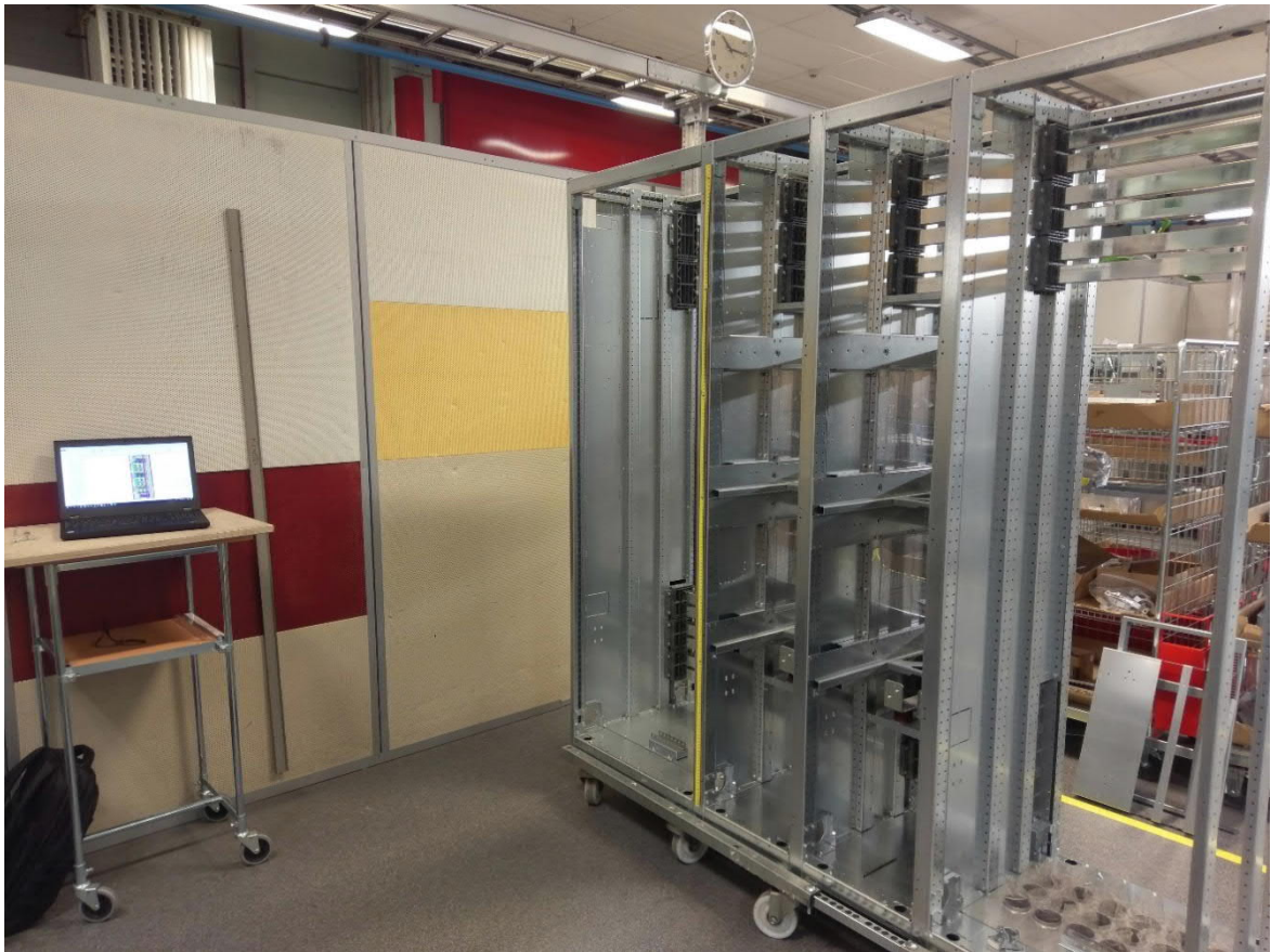
Figure 18. Picture of the mechanical assembly cell. The laptop with the 3D instructions is on the left. Test objects are the two units in the middle of the line-up.
