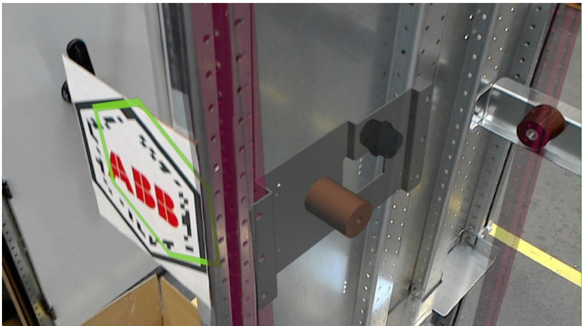
Figure 20. Bad alignment of the virtual and the physical model. The green hexagon should be aligned with the grey hexagon of the marker.
