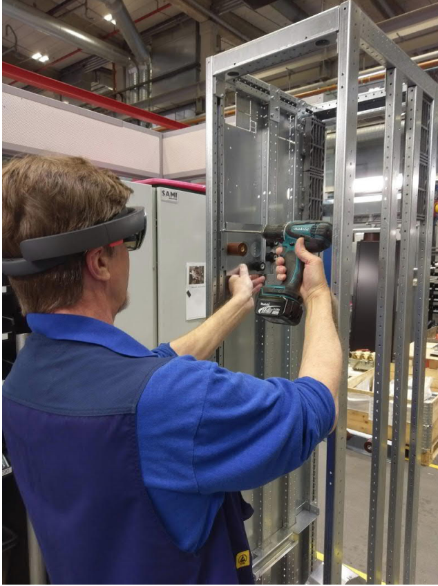
Figure 19. An operator installing support plate into the assembly object while wearing a HMD.
