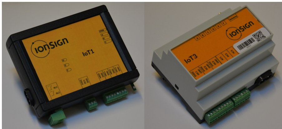
Figure 16: The second version of the switchgear sensor unit on the left and the additional sensor unit installed in a bay marshalling cabinet on the right. [46]
