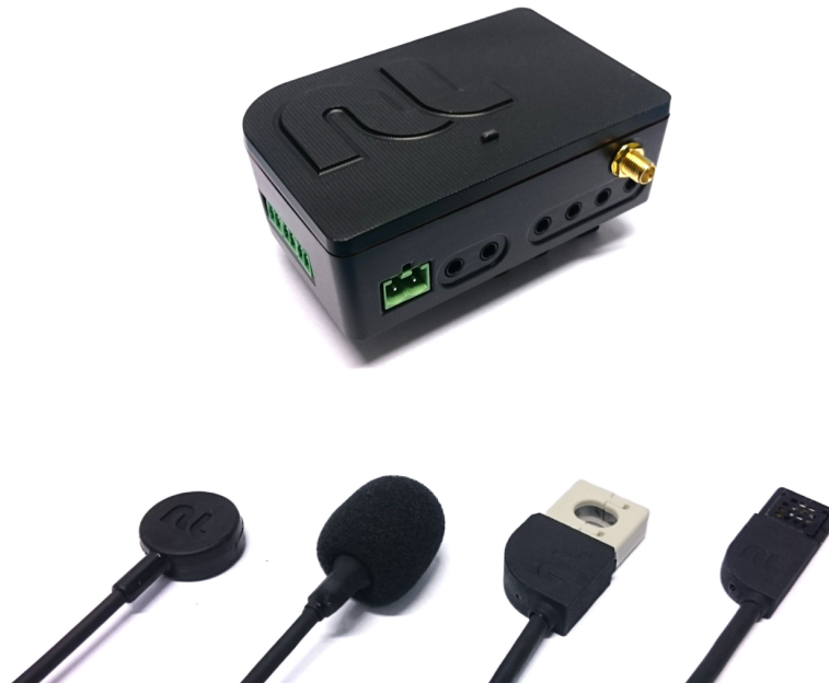
Figure 14: The first version of the IoT sensor unit for switchgear and sensors to be connected to the unit. [45]
