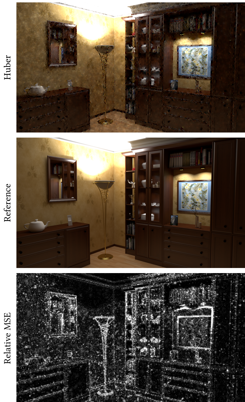
Figure 4.4: The performance of a reconstruction method is measured by its ability to produce results close to a reference image. ( Top ) 8bpp image reconstructed using Huber loss. ( Middle ) Reference image. ( Bottom ) Relative MSE measured between the reconstructed image and the reference image, darker areas indicating a lower value.
