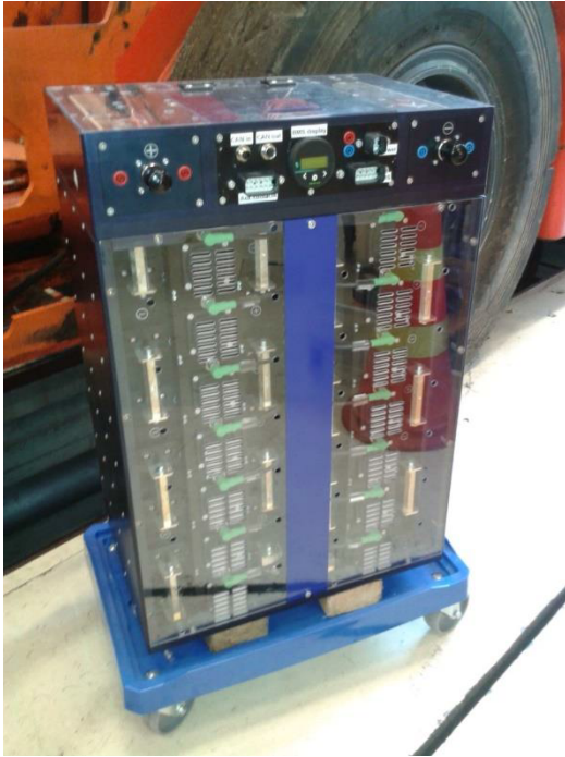
Figure 3: 362V Li-ion Aalto battery pack
