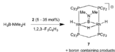
Scheme 4. Anticipated dehydrocoupling of \text{H}_3\text{B-NMe}_2\text{H} and formation of [\text{Rh}(\mu\text{-dcpm})_2(\mu\text{-H})(\mu\text{-BNMe}_2)](\text{Al}(\text{OC}(\text{CF}_3)_2)_4) ( 7 ). [\text{Al}(\text{OC}(\text{CF}_3)_2)_4]^- anion not shown.
