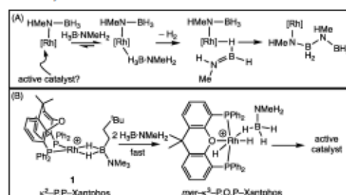
Scheme 3. (A) Proposed Coordination/Dehydrogenation/Insertion Mechanism; (B) Cationic Xantphos-Ph Precatalyst a
