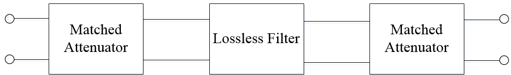
Figure 3.3: Equivalent lossy filter network with same attenuation.
