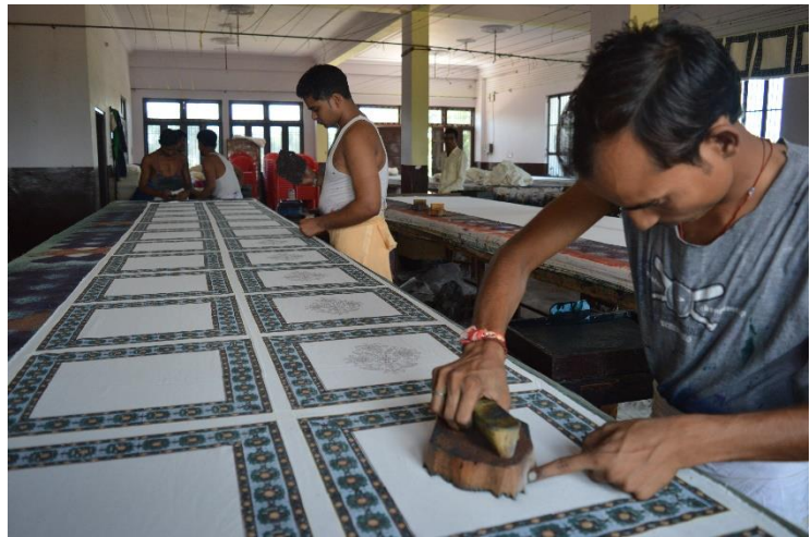
Image 18 The long tables used in present day block printing, where several workers may work together as division of labour Photo by author
