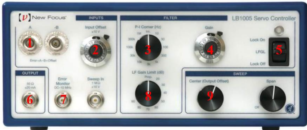
Figure 3.19: Control panel of PI amplifier (New Focus LB1005). 1, input port; 2, input offset control; 3, PI corner frequency control; 4, proportional gain control; 5, gain regime control; 6, output port; 7, error port 8, low frequency gain control; 8, output offset control.
