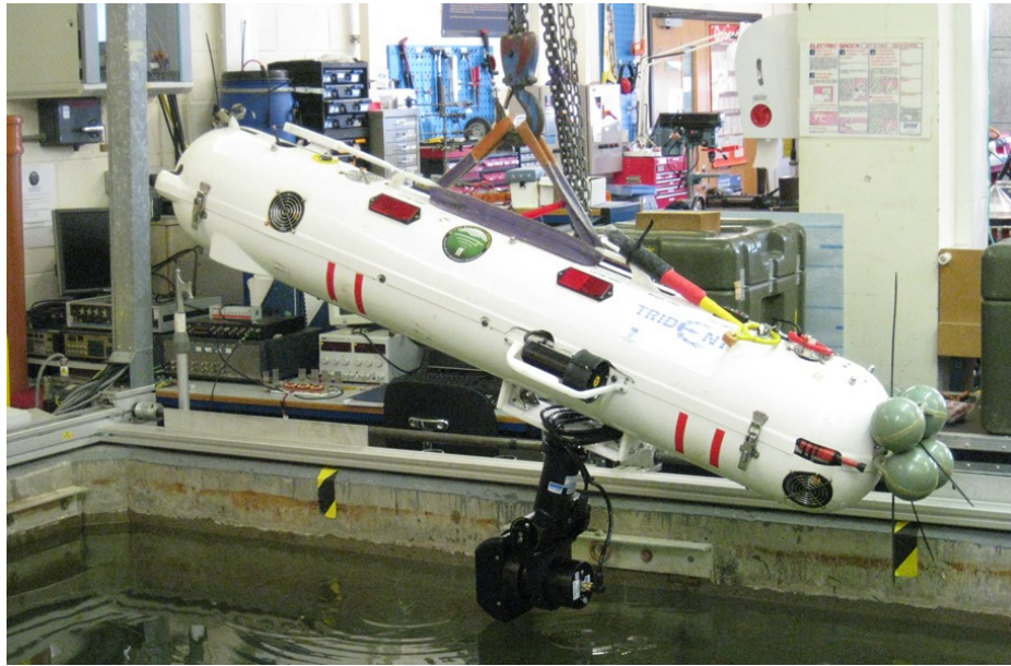
Figure 1.1: Nessie VII Ocean Systems Laboratory (OSL) main research AUV with pan and tilt sonar underneath for steering multibeam sonar.
