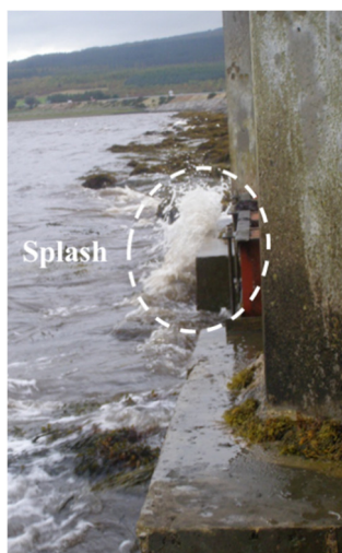
Figure 4.9 (a) Location of marine exposure site, (b) position of frames installed in XS3 environment, (c) breaking waves during the period of rising tide, and (d) retrieved samples positioned in the frame.
