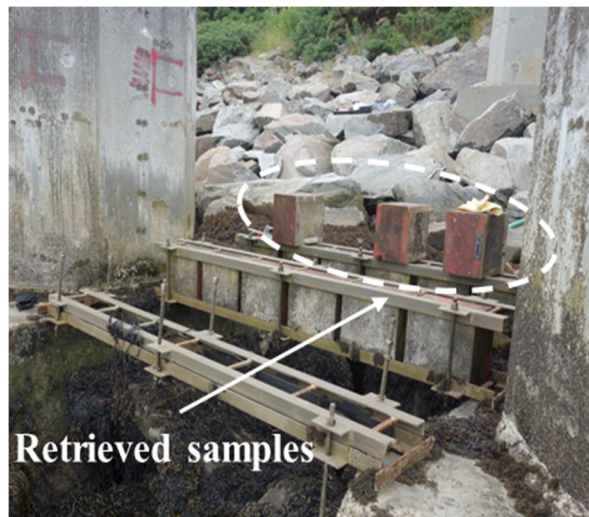
Figure 4.9 (a) Location of marine exposure site, (b) position of frames installed in XS3 environment, (c) breaking waves during the period of rising tide, and (d) retrieved samples positioned in the frame.
