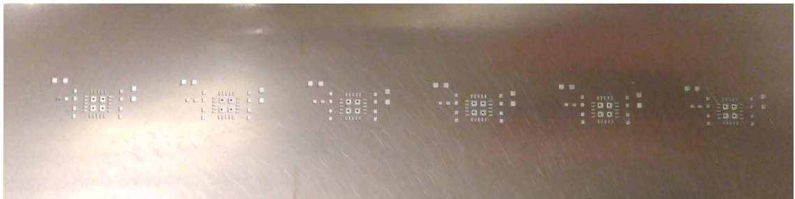
Figure 4.22: Stencil frame aligned with solder pads ready to apply the solder paste.
