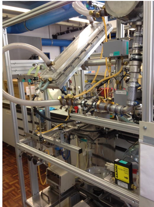
Figure 1: Sketch of the experimental set-up: a liquid film flows down the inclined channel and interacts with a counter-current gas flow.
