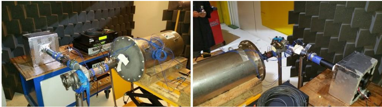
Fig. 9: Test rig for passive acoustic characterization of a static turbocharger
