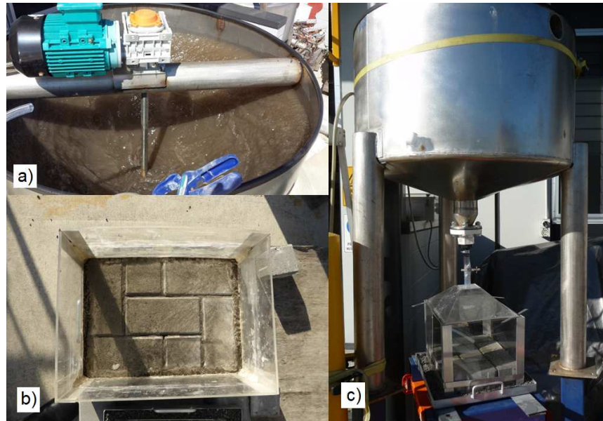
Figure 1. Accelerated Stormwater Simulation Testing Setup
