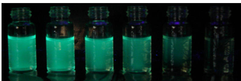
Figure 2.7. Observed luminescence quenching of 3,3'-dihydroxybipyridine upon the addition of 10^{-3} M \text{Cu}^{2+} . Source: 24
