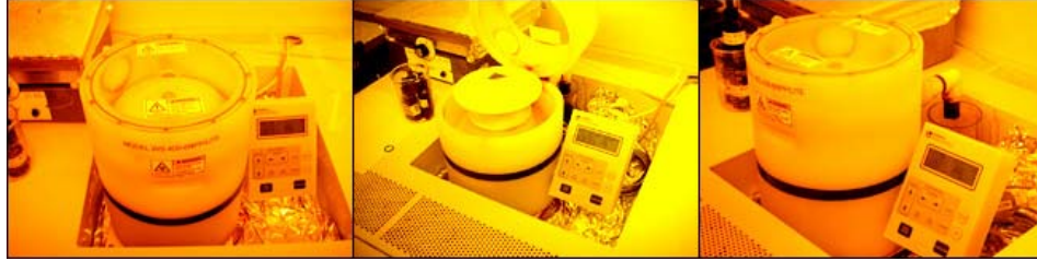
Figure 30: Laurell photoresist spinner. Courtesy of INFR centre of University of California Irvine.
