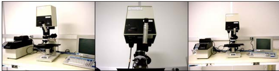
Figure 32: Nanospec thin film monitor Courtesy of INFR centre of University of California Irvine.
