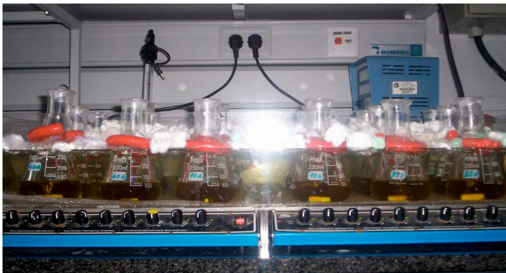
Figure 2.4. Transesterification of Cynara cardunculus oil. Experimental set-up.
