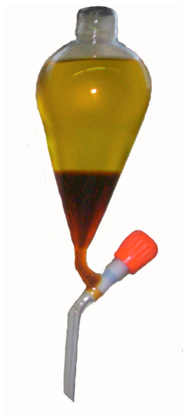
Figure 2.5. Phase separation after transesterification. Biodiesel and glycerol can be seen as the upper and lower phases respectively
