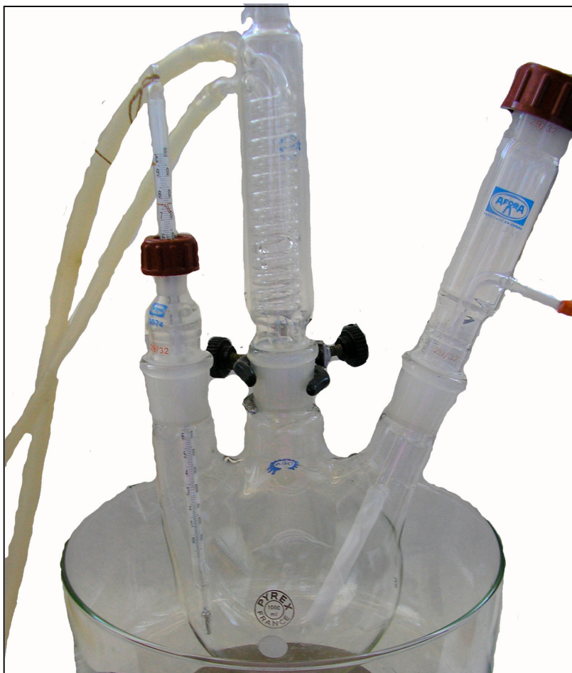
Figure 2.14. Reactor used for the transesterification of the pre-treated oil
