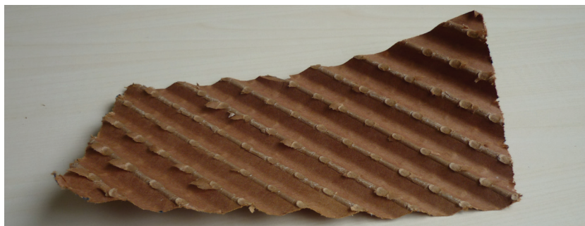
Figure 6.16 One of the sheets used to measure the volume-to-surface ratio
