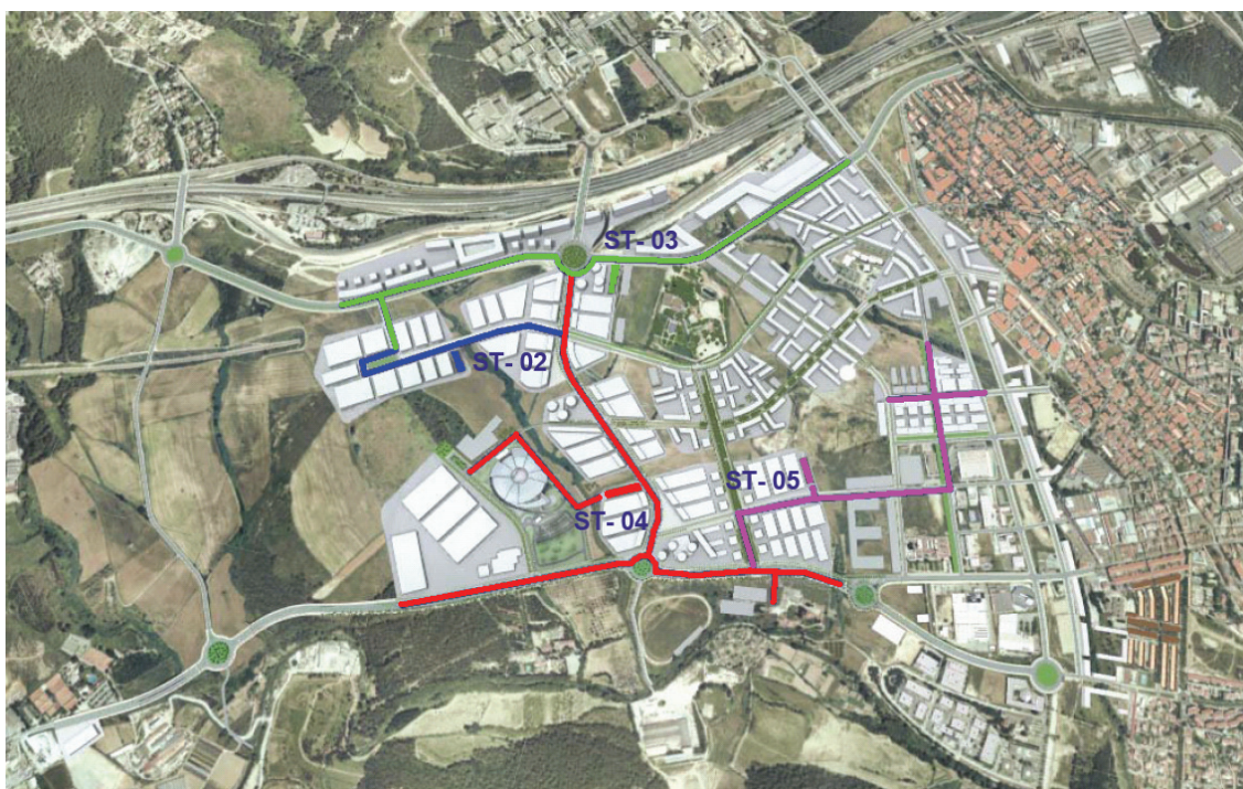
Figure 7.1 Foreseen energy supply plants and DHC network in Alba park in Cerdanyola del Vallès
