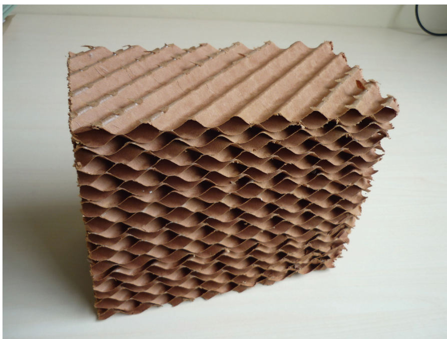
Figure 6.14 Cellulose packet used in the dehumidifer and regenerator columns
