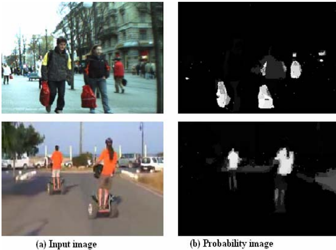
Figure 7 Two examples of probability images given by neural network method in the static recognition module.
