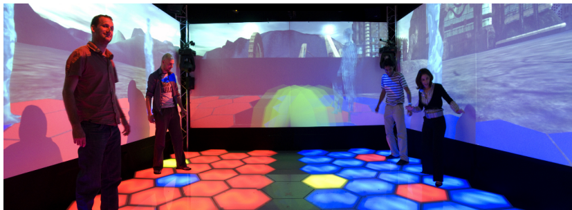
Figure 4.2: XIM Multiuser Interaction Scenario: Multiple real users interacting with each other in a mixed reality Pong game, which is one of the scenarios used to evaluate PASAR performance. Also remote users take part in the same interaction by logging in from remote machines into the virtual world and they are represented by avatars on the projection screens (adapted from [55]).
