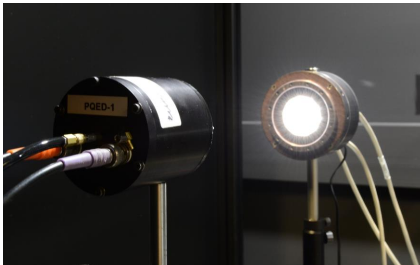
Figure 4 – Illuminance measurement of the luminous intensity LED standard lamp LIS-A using unfiltered Predictable Quantum Efficient Detector (PQED) with nitrogen flow.
