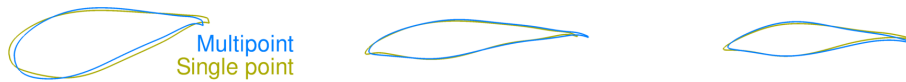
Figure 18. Comparison of airfoil profiles obtained from single-point and multipoint optimizations. The profiles are taken from 35, 64, and 84 m spanwise positions.
