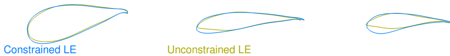
Figure 19. Comparison of airfoil profiles obtained from multipoint optimizations with and without LE geometric constraint.
