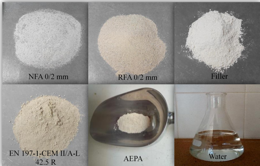
Figure 5. Components of masonry mortars
