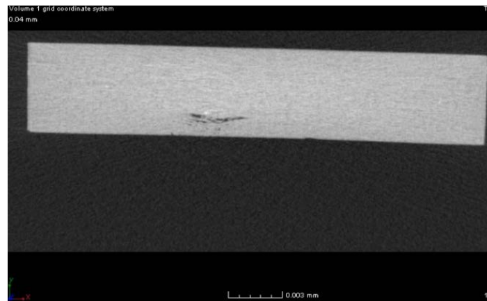
Figure 4. Typical Micro-CT image of discontinuous PEEK/CF composite
