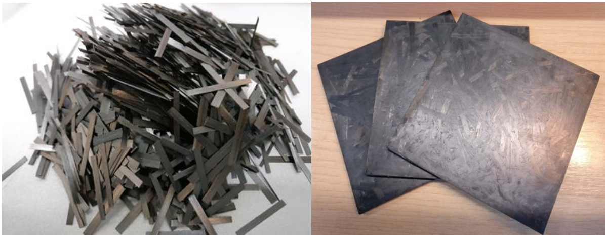
Figure 1. Discontinuous PEEK/CF tapes and the resulting compression moulded composite panels.
