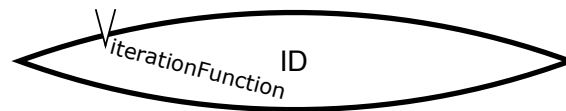
Figure 5.3. The central ID node. We start with a central ID node (one which provides its sole input, unaltered, as an output) with an input named ‘iterationFunction’.
