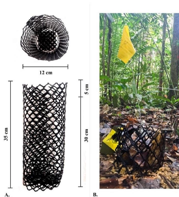
Figure 4.2. Detail of the ingrowth core and its dimensions on the left panel; ingrowth core installed in the field in the right panel. Photo credit: J. S. Rosa.
