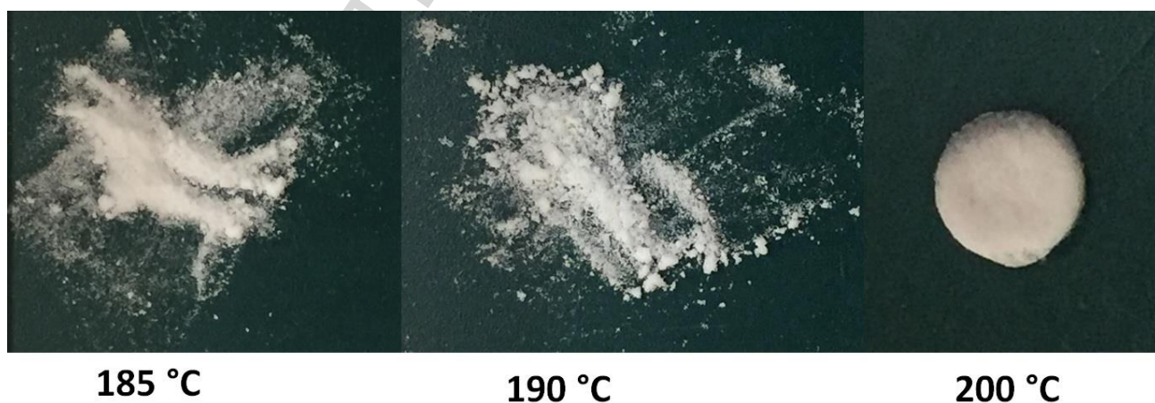
Figure 10. PA1101 powder heated from room temperature to 185, 190 and 200 °C using DSC
