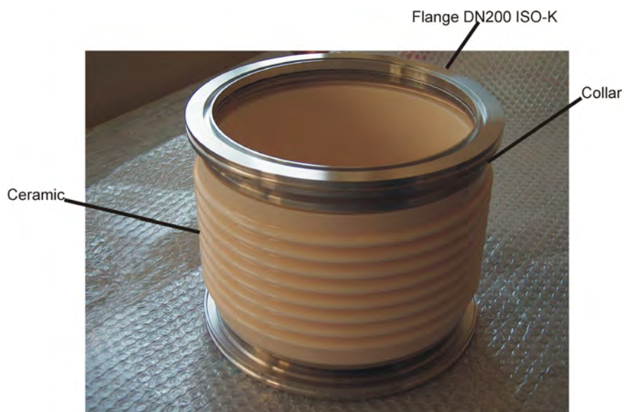
Figure 8.5: Picture of a high voltage ceramic insulator
