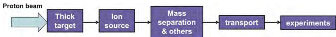
Figure 1.4: Scheme of the procedure to produce and transport RIB's at ISOL facilities
