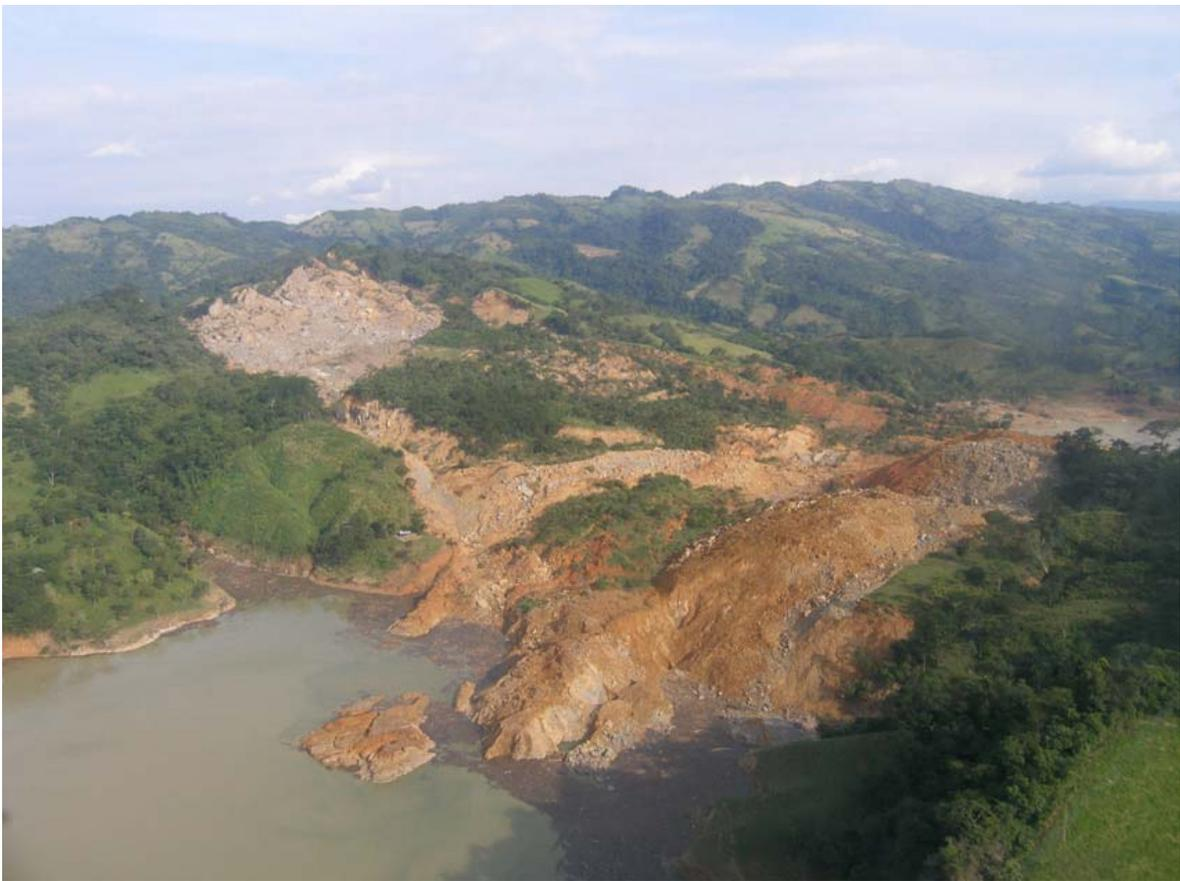
Figure 1.11 San Juan de Grijalva landslide blocking the river (Alcántara-Ayala *et al.*, 2008).
