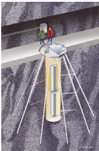
Figure 6.2. Principle design of the Temperature Buffer Test (SKB, 2005).
