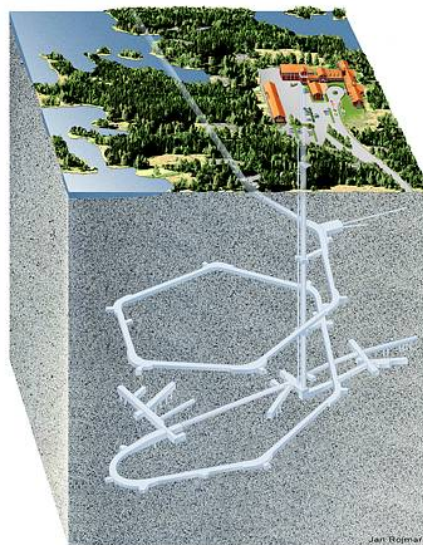
Figure 6.1. General layout of the Äspö Hard Rock Laboratory ( http://www.skb.se ).
