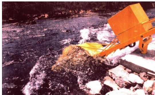
Figure 3. Fully submerged turbine in the river was hold by a long lever at the river bank [17].
