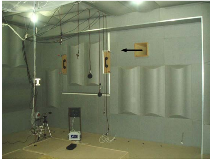
Figure 3.2: Semianechoic room and tube output signal (arrow)
