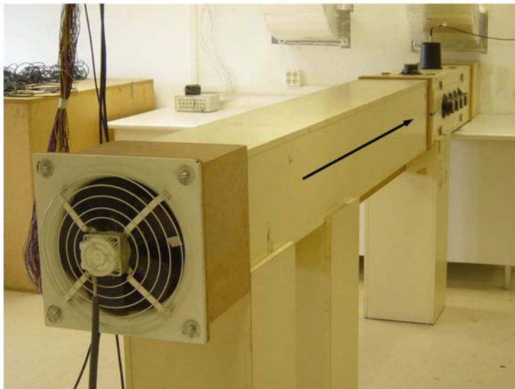
Figure 3.1: Tube and input noise source (fan)
