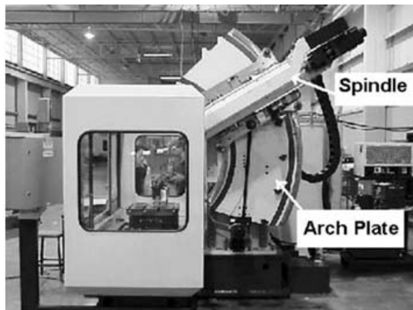
Figure 2.1: Full scale prototype of Arch-Type RMT (Katz, 2007)
