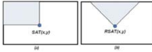
Figure 2.31: Definition of (a) Summed Area Table (SAT) (b) Rotated Summed Area Table (RSAT) .
