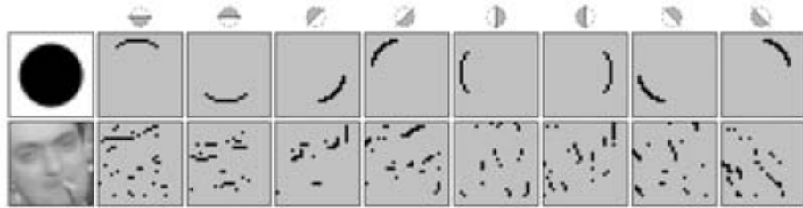
Figure 2.10: The original gray-scale pictures are shown on the left. The eight binary maps on the right show the responses of the edge detectors at every locations in the 28 \times 28 frame, for every one of the 8 possible directions and polarities. The binary features are disjunctions of such edge detectors in small neighborhoods, which ensure their robustness to image deformations [Fle04].
