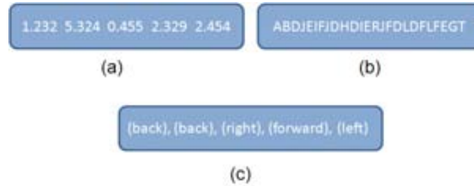
Figure 3.6: Codification using value encoding. (a) Real values (b) Char strings (c) Movements sequence.
