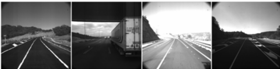
Figure A.2: Some examples of images acquired by Geomobil system. From left to right, we see a normal illuminated image, effect of road artifacts (bridge), light image and dark image.
