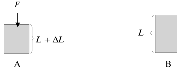
Figure 3.1 Force and loading: A. Material bar being loaded; B. unloaded bar.
