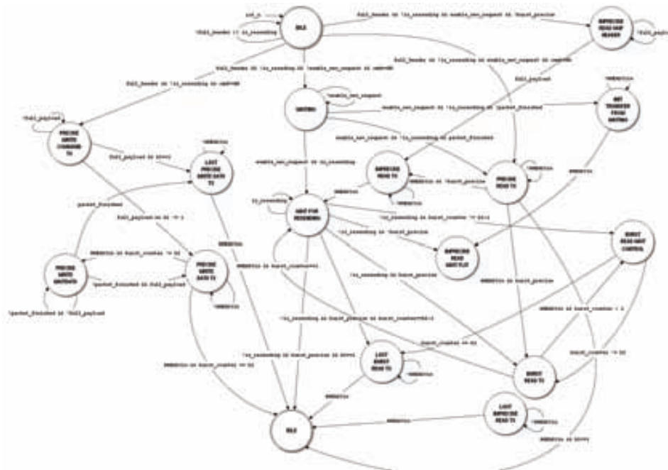
Figure 3.8: AMBA 2.0 AHB NI receive FSM
