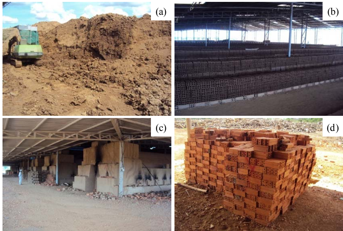
Figure 2.6: Procedures of making bricks in Kandal: (a) raw clay; (b) drying of extruded green body; (c) firing kiln and (d) fired bricks
