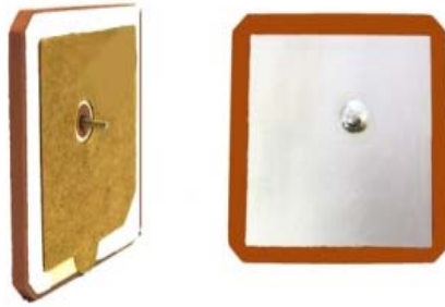
Figure 2.2 Microstrip patch antenna for GPS application (Maxtena, 2009)
