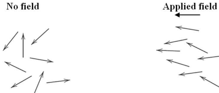
Figure 2.4: Response of permanent electric dipoles (arrows) to an applied electric field, producing orientation polarization (Wyatt and Hughes, 1974).
