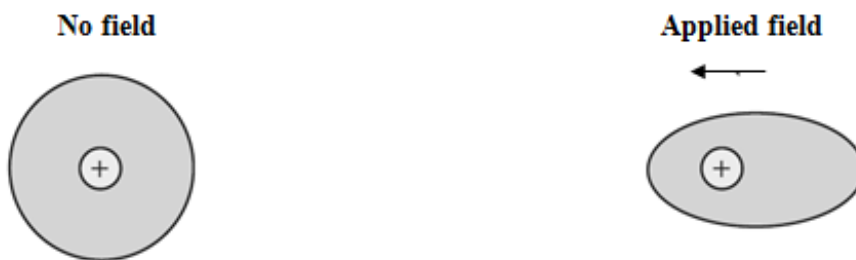
Figure 2.2: Electronic polarization that results from the distortion of an atomic electron cloud by an electric field (Wyatt and Dew-Hughes, 1974).
