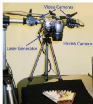
Figure 2.6: 3D scanning system (Brown et al., 2007).
