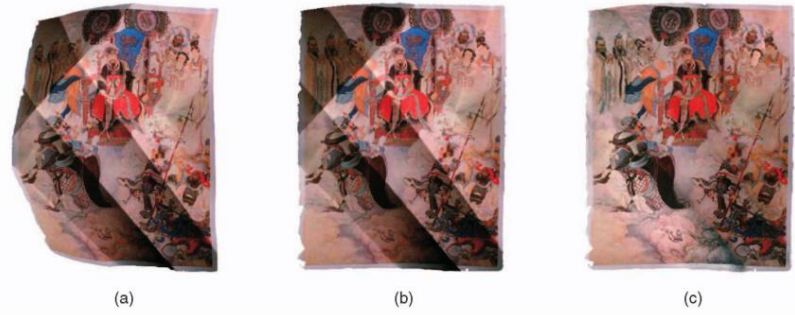
Figure 2.4: (a) Original image exhibiting geometric and illumination distortion. (b) Geometry corrected. (c) Geometry and illumination corrected (Brown et al., 2007).
